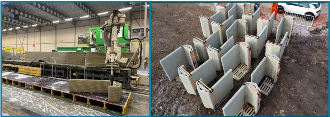
Figure 13: 3D concrete printing in action (left); the finished product (right)
